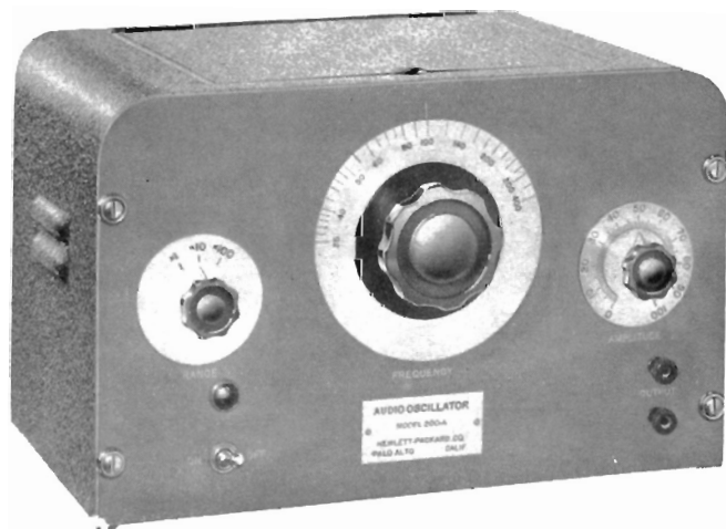
Here's the first -hp- electronic test instrument, the Model 200A resistance capacity audio oscillator that established new performance and value standards for this basic type of laboratory equipment. A number of these instruments produced fifteen years ago are still in operation.
